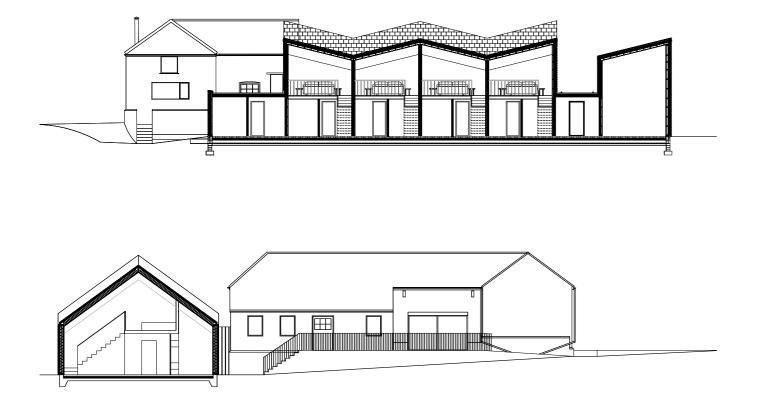
Longitudal and cross sections, showing sleeping areas on the upper level. Shelves, displaying an array of beautiful design objects are placed between the entrance doors to the rooms.
